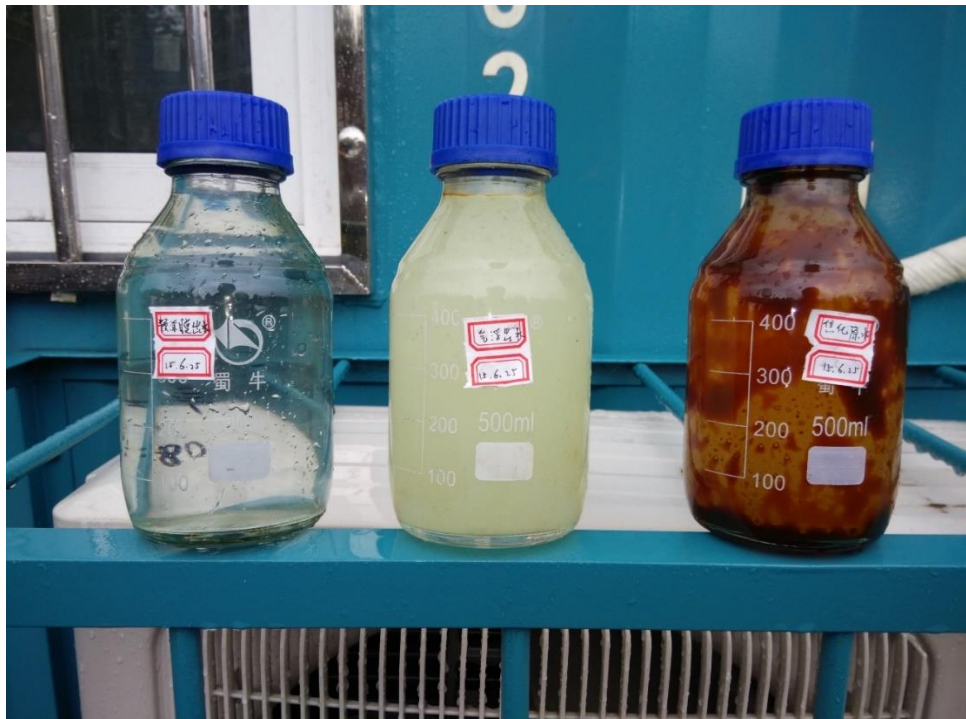
Photo 1: This is a raw water sample from a refinery coker wastewater which is first treated with a flotation technology. The middle sample is the effluent from the flotation technology. Note the cloudy appearance of the water. The cloudy appearance is due to emulsified oil and colloidal solids. RSL Membranes™ removed the oil and particle colloids. The permeate is the left sample.
